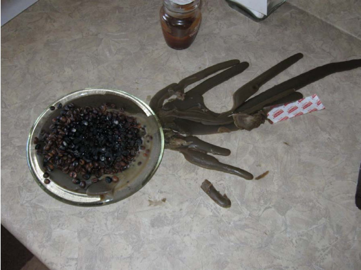
Figure 1 - This photo shows the remains of a candle on a glass candle holder. The candle contained coffee beans on both the inside and the outside of the candle. The photo shows how the coffee beans ignited and the wax poured onto the kitchen counter.
